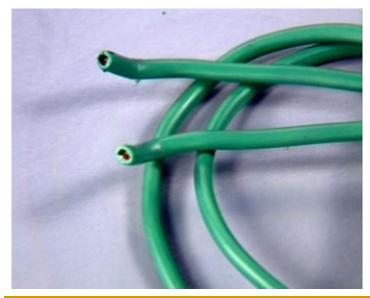
Conductor = Copper Wire Insulator = Plastic sheath
