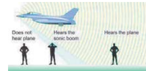
Figure 21.4: If a supersonic jet flew overhead, you would not hear the sound until the plane was far beyond you. The boundary between sound and silence is called a “shock wave.” It is almost as if all the sound were compressed into a thin layer of air. The person in the middle hears a sonic boom as the shock wave passes over him. Because the sonic boom can shatter windows, planes are not allowed to fly over cities at supersonic speeds.
