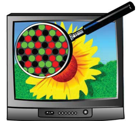
Figure 22.17: A television makes colors using tiny glowing dots of red, green, and blue.
