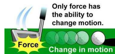
Figure 2.1: Force is the action that has the ability to change motion. Without force, the motion of an object cannot be started or changed.
