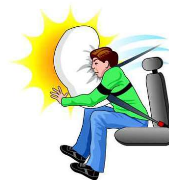
Figure 3.20: Seat belts and air bags work together to safely stop passengers in automobile collisions.
