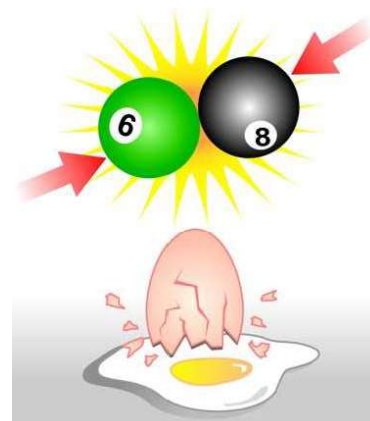
Figure 3.16: The collision of two billiard balls is elastic. The collision of an egg with the floor is inelastic.
