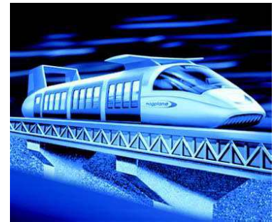
Figure 5.19: With a maglev train, there is no contact between the moving train and the rail — and thus little friction.
