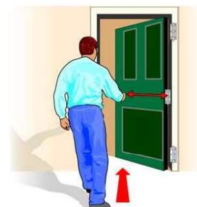
Figure 5.22: A door rotates around its hinges and a force creates the greatest torque when the force is applied far from the hinges.
