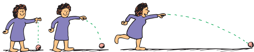
◀ FIGURE 14.1 The greater the stone's horizontal motion when released, the wider the arc of its curved path.
