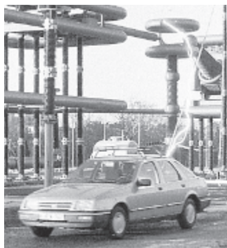
FIGURE 33.6 ▲ Electrons from the lightning bolt mutually repel and spread over the outer metal surface. The overall electric field inside the car practically cancels to zero.
