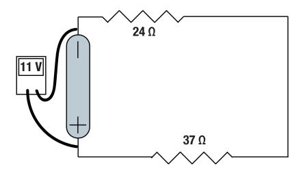
$$R_{eq} = R_{24\Omega} + R_{37\Omega}$$
