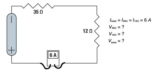
a. voltage drop across the 35  $\boldsymbol{\Omega}$  resistor
