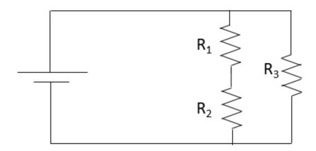
$$R_{1+2} = R_1 + R_2$$
