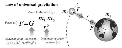
So, when the masses  $m_1$  and  $m_2$  are given in kilograms and the distance *r* is given in meters, the force has the unit of newtons. Remember that the distance *r* corresponds to the distance between the center of gravity of the two objects.
